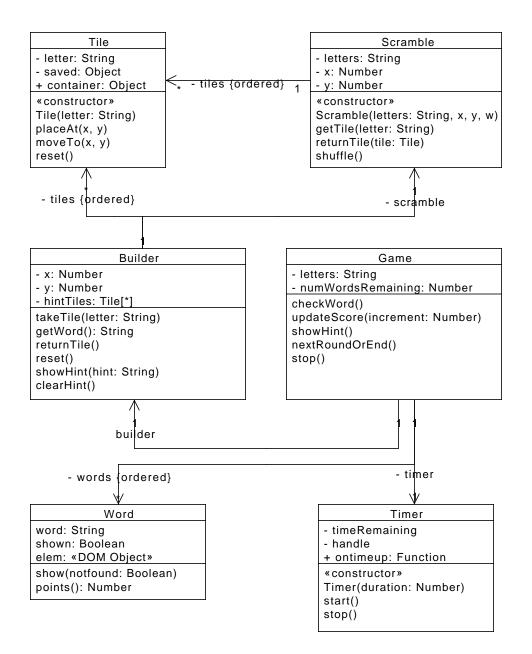
**Figure 3:** A class diagram showing the classes that make up the Letter Lizard JavaScript implementation. The event-driven, callback-based client-side scripting environment naturally led to a modularized, class-based design for this implementation.
